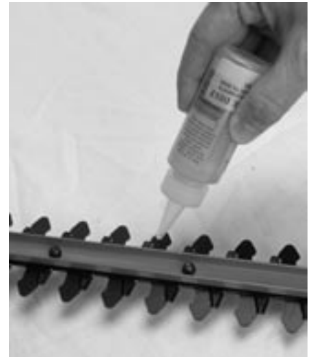
Figure 4-3 : Lubrification des lames
